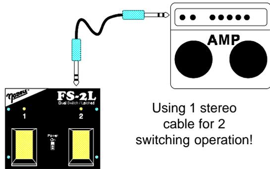
Using 1 stereo cable for 2 switching operation!
