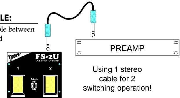
Using 1 stereo cable for 2 switching operation!
