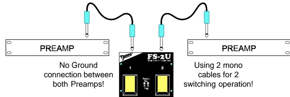
No Ground connection between both Preamps!
