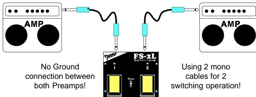
No Ground connection between both Preamps!
